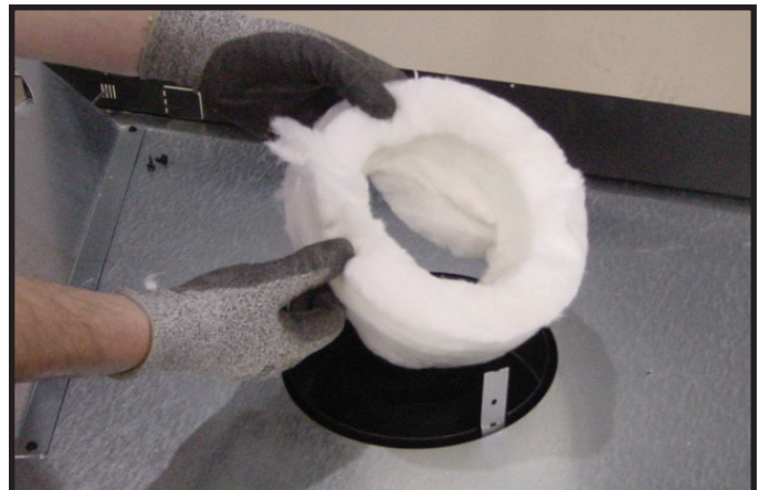
Figure 7.6 Remove the insulation from the outer vent pipe. For rear venting there is no insulation in the outer vent pipe. Replace the top heat shield.
